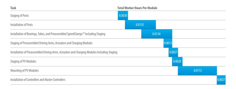
Modules: Polysilicon framed modules 380 Watts Site Conditions: Flat to slightly rolling topography Wind: 105 mph ASCE-10 Snow: 5 psf
