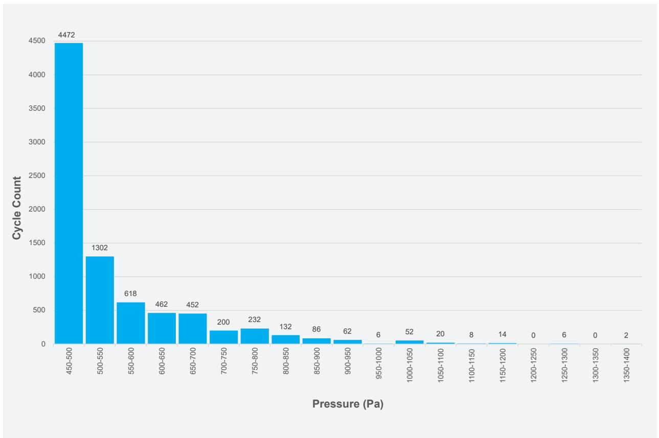
**FIGURE 3:** CPP Analysis Pressures on Module Leading Edge vs Cycle Counts for Sample Site During Hurricane Ian
